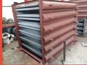
Tea Dryer Steam Radiators
