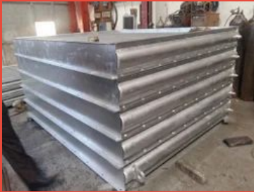
Tea Dryer Steam Radiators
