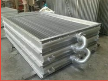
Thermic Fluid Heat Exchanger for Sago Industries
