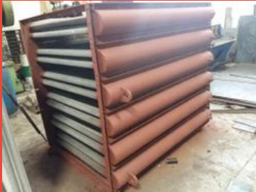
Rice Mills Heat Exchanger
