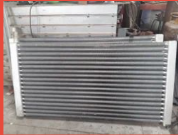
Air Cooled Oil Coolers
